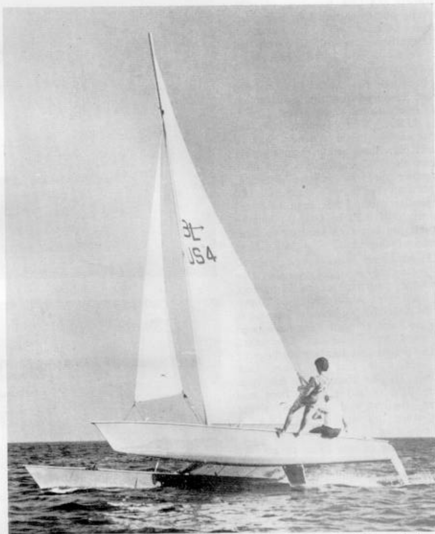
B-Lion an American International B class catamaran designed by the Hubbard brothers and built in fibreglass by the American Fibreglass Corporation. The B class has not yet proved as popular as the A and the C classes
