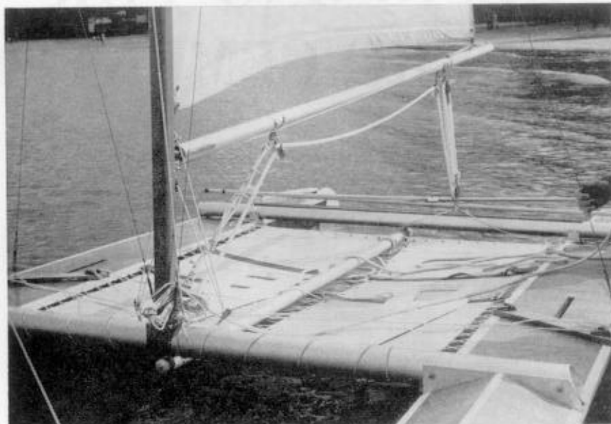
Rascal's deck is terylene cloth. The sail is loose footed with a foot batten. The hull decks are flat amidships and peaked for'ard of the fore-beam
