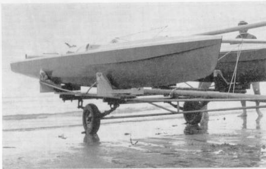
Rascal on her trailer showing the very fine entry and the knuckle in the topsides for'ard
