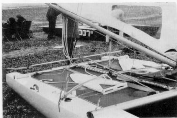
TOP: Here Mazzotti sits well aft to trim Unicorn on a reach—weather dagger board is well lifted. Notice the pronounced bend in the mast even with the boat off the wind.
